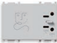
14290.SL 230 V~ 50/60 Hz, with 20 VA isolating transformer, 230 V~ and 120 V~ outputs - 3 modules. Depth: 41 mm
