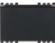
19453 Transponder card reader, vertical pocket for inside the room, KNX standard, 2 relay outputs NO 4 A 24 V~, 2 inputs, 12-24 V~ 50/60 Hz and 12-24 V D.C. (SELV), grey - 3 modules. Depth: 37 mm
