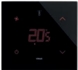
21814.F.76 Touch screen thermostat (heating and air conditioning), 3-speed and proportional FAN COIL control, class I (contribution 1%) in ON/OFF mode, class IV (contribution 2%) in PID mode, can be interfaced with actuator 01466.1 to make a class V modulating room thermostat (contribution 3%), 1 input for sensor 20432, 19432 or 14432 or wired sensor 02965.1, 1 programmable digital input, RGB LED backlighting, black diamond - 2 modules. Depth: 30,2 mm
