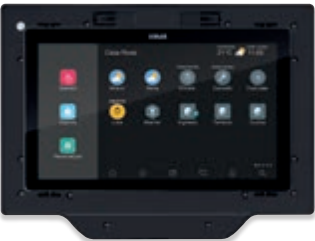
01425 Colour 10" IP touch screen, used as a home automation system supervisor, IP/Due Fili Plus video door entry indoor station, IP video camera and CCTV system manager, PoE or 12-30 VDC, surface mounting with bracket on round mounting box, 3 module rectangular (horizontal and vertical), 8 module (4+4) and BS square mounting box, black
