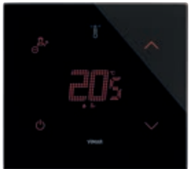
21814.H.76 Touch screen thermostat (heating and air conditioning), MAKE UP ROOM and DO NOT DISTURB control, class I (contribution 1%) in ON/OFF mode, class IV (contribution 2%) in PID mode, can be interfaced with actuator 01466.1 to make a class V modulating room thermostat (contribution 3%), 1 input for sensor 20432, 19432 or 14432 or wired sensor 02965.1, 1 programmable digital input, RGB LED backlighting, black diamond - 2 modules. Depth: 30,2 mm
