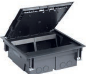
V54420.01 Floor mounting retractable turret with stainless steel cover for Eikon, Arké and Plana devices for installation on floating floors. Supplied with 2 mounting frames with 6 modules. Installation in screed with dedicated mounting box V54920
