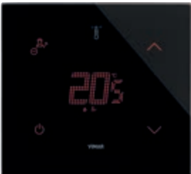
21514.H.76 Touch screen thermostat (heating and air conditioning), MAKE UP ROOM and DO NOT DISTURB control, class I (contribution 1%) in ON/OFF mode, class IV (contribution 2%) in PID mode, can be interfaced with actuator 01466.1 to make a class V modulating room thermostat (contribution 3%), 1 input for sensor 20432, 19432 or 14432 or wired sensor 02965.1, 1 programmable digital input, RGB LED backlighting, black diamond - 2 modules. Depth: 30,2 mm
