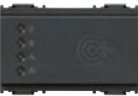
16927 Transponder card reader for outside the room, KNX standard, 2 relay outputs NO 4 A 24 V~, 2 inputs, 12-24 V~ 50/60 Hz and 12-24 V D.C. (SELV), grey - 3 modules. Supplied without transponder card. Depth: 36.5 mm
