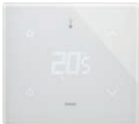
21814.S.70 Touch screen thermostat (heating and air conditioning), configurable STAR control, class I (contribution 1%) in ON/OFF mode, class IV (contribution 2%) in PID mode, can be interfaced with actuator 01466.1 to make a class V modulating room thermostat (contribution 3%), 1 input for sensor 20432, 19432 or 14432 or wired sensor 02965.1, 1 programmable digital input, RGB LED backlighting, white diamond - 2 modules. Depth: 30,2 mm
