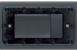
20450 Transponder card reader/ programmer in 4-module tilted table mounting box, grey. To be completed with Eikon 4-module cover plate. Dim.: 148.6x79x9x88.8 mm
