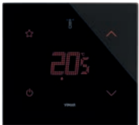
21814.S.76 Touch screen thermostat (heating and air conditioning), configurable STAR control, class I (contribution 1%) in ON/OFF mode, class IV (contribution 2%) in PID mode, can be interfaced with actuator 01466.1 to make a class V modulating room thermostat (contribution 3%), 1 input for sensor 20432, 19432 or 14432 or wired sensor 02965.1, 1 programmable digital input, RGB LED backlighting, black diamond - 2 modules. Depth: 30,2 mm
