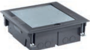
V54420 Floor mounting retractable turret with hollow cover for Eikon, Arké and Plana devices for installation on floating floors. Supplied with 2 mounting frames with 6 modules. Installation in screed with dedicated mounting box V54920
