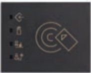
30567.G Transponder card reader for outside the room, KNX standard, 2 relay outputs NO 4 A 24 V~, 2 inputs, 12-24 V~ 50/60 Hz and 12-24 VDC (SELV), black - 3 modules. Supplied without transponder card. Depth: 38.8 mm
