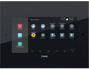
01422 Colour 7" IP touch screen, used as a home automation system supervisor, IP/Due Fili Plus video door entry indoor station, IP camera and CCTV system manager, PoE or 12-30 VDC, surface mounting with bracket on round mounting box, rectangular 3 module (horizontal and vertical), 8 module (4+4) and BS square mounting box, black
