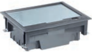
V54412 Floor mounting retractable turret with hollow cover for Eikon, Arké and Plana devices for installation on floating floors. Supplied with 2 mounting frames with 6 modules. Installation in screed with dedicated mounting box V54912
