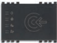
19457 Transponder card reader for outside the room, KNX standard, 2 relay outputs NO 4 A 24 V~, 2 inputs, 12-24 V~ 50/60 Hz and 12-24 V D.C. (SELV), grey - 3 modules. Supplied without transponder card. Depth: 37 mm
