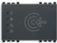
20457 Transponder card reader for outside the room, KNX standard, 2 relay outputs NO 4 A 24 V~, 2 inputs, 12-24 V~ 50/60 Hz and 12-24 V D.C. (SELV), grey - 3 modules. Supplied without transponder card. Depth: 37 mm
