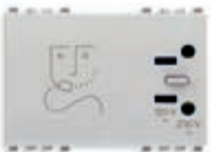
20290.N 230 V~ 50/60 Hz, with 20 VA isolating transformer, 230 V~ and 120 V~ outputs - 3 modules. Depth: 42 mm
