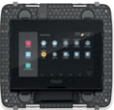
01420 Colour 4.3" IP touch screen, used as a home automation system supervisor, IP/Due Fili Plus video door entry indoor station, IP camera and CCTV system manager, PoE or 12-30 VDC, complete with mounting frame for flush mounting in 8 module boxes (4+4), to completed with Eikon, Arké or Plana cover plates, black
