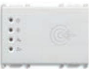
14457 Transponder card reader for outside the room, KNX standard, 2 relay outputs NO 4 A 24 V~, 2 inputs, 12-24 V~ 50/60 Hz and 12-24 VDC (SELV), white - 3 modules. Supplied without transponder card. Depth: 36 mm
