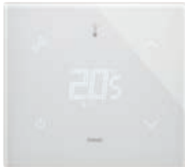
21514.H.70 Touch screen thermostat (heating and air conditioning), MAKE UP ROOM and DO NOT DISTURB control, class I (contribution 1%) in ON/OFF mode, class IV (contribution 2%) in PID mode, can be interfaced with actuator 01466.1 to make a class V modulating room thermostat (contribution 3%), 1 input for sensor 20432, 19432 or 14432 or wired sensor 02965.1, 1 programmable digital input, RGB LED backlighting, white diamond - 2 modules. Depth: 30,2 mm
