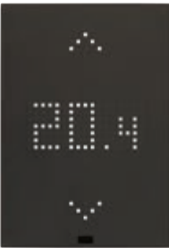
32041.G XT thermostat for By-me Plus home automation system for room temperature control (heating and air conditioning), 2- and 4-pipe system management, 3-speed and proportional fan coil control, class I temperature control device (contribution 1%) in ON/OFF mode, class IV (contribution 2%) in PID mode, can be interfaced with actuator with proportional analogue outputs 01466.1 to make a class V modulating room thermostat (contribution 3%), boost function to activate a second source, proximity function, LED backlighting, black - 2 front modules
