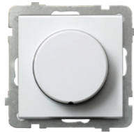
ŁP-8RL2/m/00 2006 Universal dimmer load: GLS – 10-250W, CFL – 5-75W LED – 0-100W functions: electronic switch, "time to bed"
