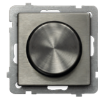
ŁP-8RML2/m/37 Universal dimmer load: GLS – 10-250W, CFL – 5-75W LED – 0-100W functions: electronic switch, “time to bed” 1179
