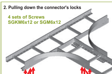
Assembly Example of Add-one Connector LDDKP2 in Combination with Cable Ladder Lengths Joined through Corner Connector LKUC2
