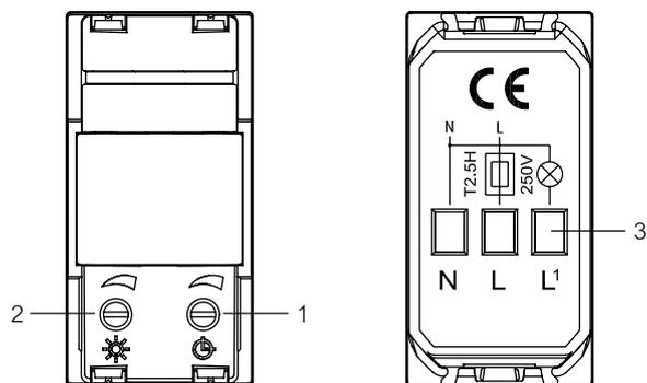
1. Switching off delay adjustment (\*)
