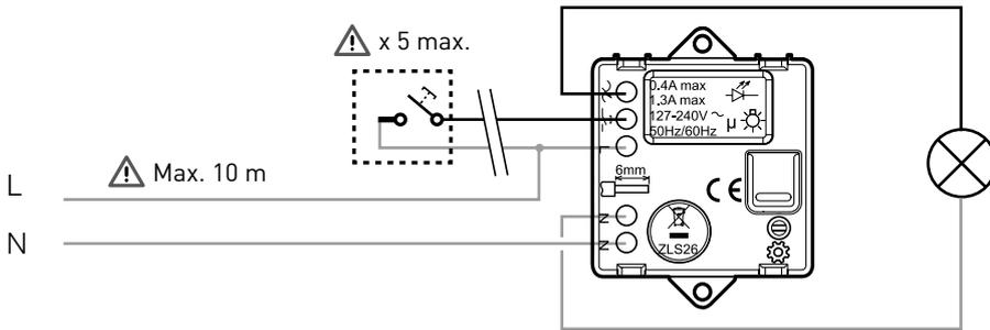
Option: remote control through mechanical pushbutton, not luminous.
