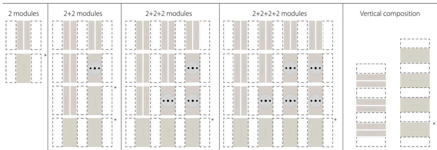
\* **Note:** for solutions using one 2-module cover for the main controls, it will be necessary to use two "half-module blanking modules" (item K4949) at the sides of the control. (see the sample diagrams below)
