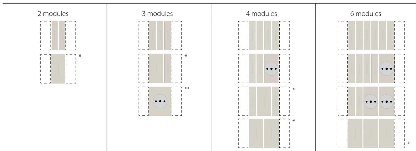
\* **Note:** for solutions using one 2-module cover for the main controls, it will be necessary to use two "half-module blanking modules" (item K4949) at the sides of the control. (see the sample diagrams below)
