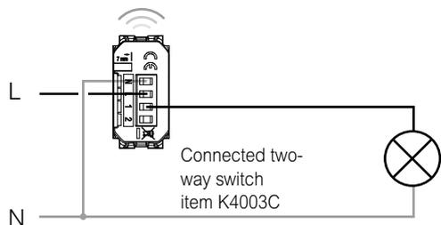
Wiring diagram - redirected or inverted
