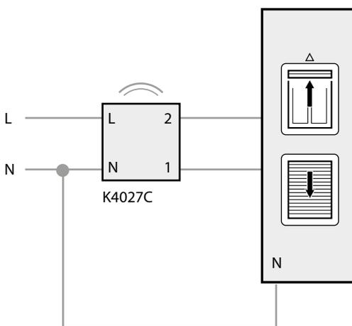
Warning: only compatible with standard motors (no pulse motors, no radio motors)
