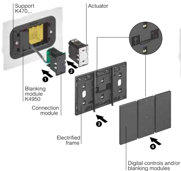
Use in conjunction with the connection module, or another actuator, to take up the power voltage.
