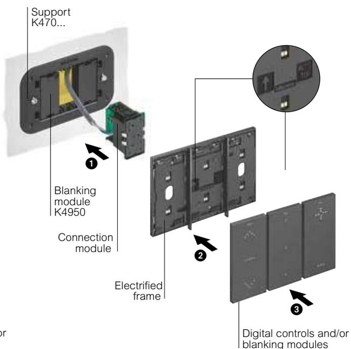
At the side of the connection module, install 2 false poles, item K4950, in any position.
