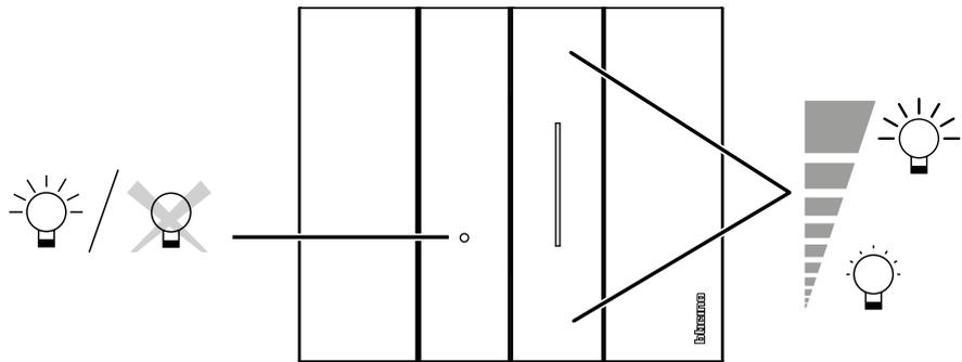
Switch the light on and off and bring the light to the desired level with a simple soft touch.
