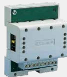
Individual protection device which makes it possible to isolate and identify short circuits on the bus line. Equipped with 4 LEDs, one for each output, it locates the problem immediately. When used in conjunction with the porter switchboard, the mixer and the riser distributor (1414), it offers complete protection.
