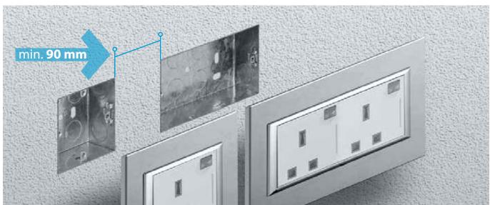
For a correct AXOLUTE cover plates installation on flush mounting boxes BTicino recommends that the minimum distance between boxes, both square (72x72) and rectangular (72x135) must be 90 mm
