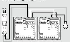
The IR sensor of the two switches are both activated when the light is switched on. The light will switch off when one of the two switches stays 10 minutes with no movement detection.
