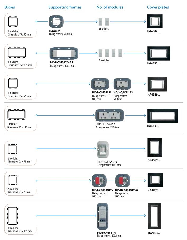
**NOTE:** before installing boxes, check plate dimensions (see pages Dimensional data) Devices available in white, tech and athracite colour.
