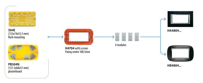
**NOTE:** the supporting frames are supplied with a pre-installed orange frame-cover and a transparent protection. It is recommended to remove the frame-covers before installing the plates. Devices available in white, tech and athracite colour.
