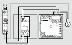
The IR sensor is activated when the light is switched on from one of the two switches. The tw-way energy saving can be installed both near or far from the load and it opens the circuit after 10 minutes with no movement detection.
