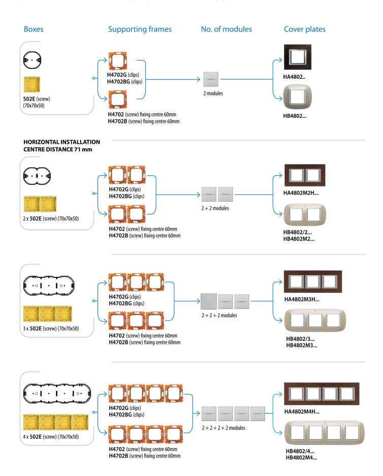
**NOTE:** the supporting frames are supplied with a pre-installed orange frame-cover and a transparent protection. It is recommended to remove the frame-covers before installing the plates. Devices available in white, tech and athracite colour.
