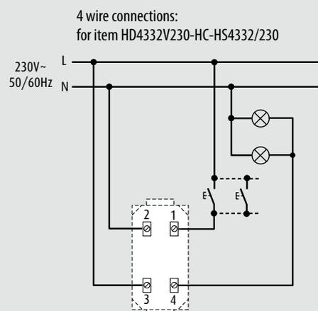
\*\* Light bulb cannot be installed with item HD4332V230-HC-HS4332/230
