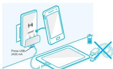
For wireless induction charging of devices fitted with suitable receivers. Also has a USB 2,400 mA socket
