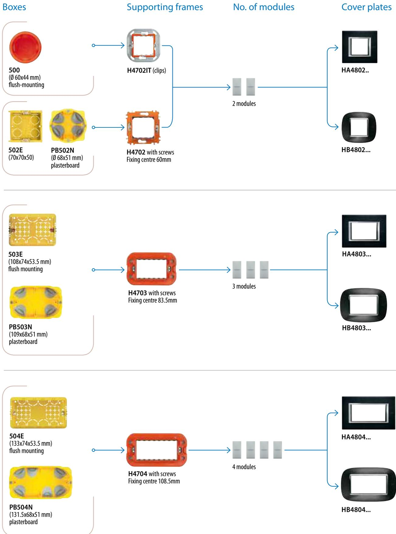
**NOTE:** the supporting frames are supplied with a pre-installed orange frame-cover and a transparent protection. It is recommended to remove the frame-covers before installing the plates. Devices available in white, tech and atracite colour.
