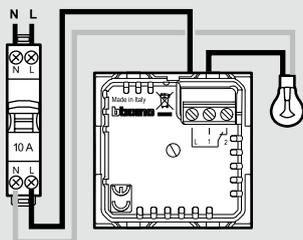
**Two-way switch + Two-way energy saving switch**
