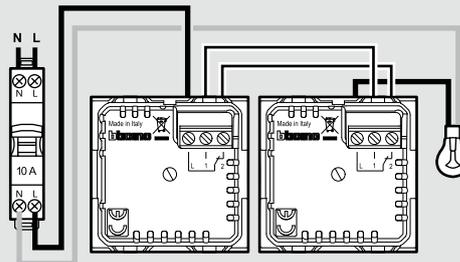
The IR sensor of the two switches are both activated when the light is switched on. The light will switch off when one of the two switches stays 10 minutes with no movement detection.
