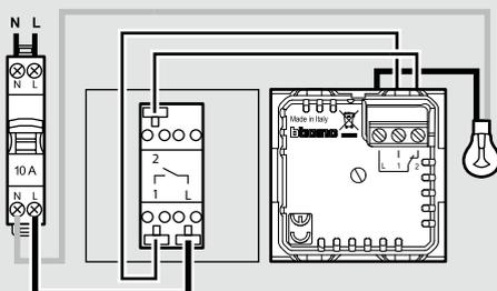
The IR sensor is activated when the light is switched on from one of the two switches. The two-way energy saving can be installed both near or far from the load and it opens the circuit after 10 minutes with no movement detection.
