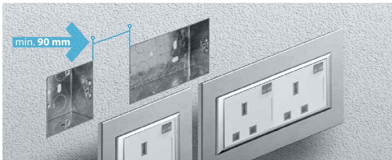
For a correct AXOLUTE cover plates installation on flush mounting boxes BTicino recommends that the minimum distance between boxes, both square (72x72) and rectangular (72x135) must be 90 mm
