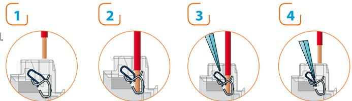
After stripping the cable, put it directly into the terminal      Use a screwdriver to pull out the cable
