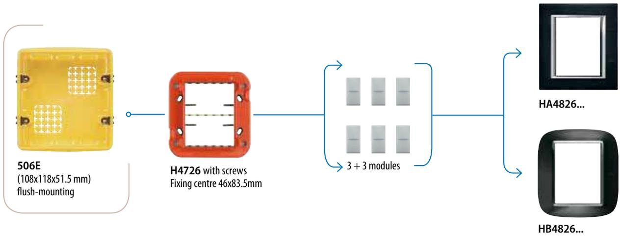
**NOTE:** the supporting frames are supplied with a pre-installed orange frame-cover and a transparent protection. It is recommended to remove the frame-covers before installing the plates. Devices available in white, tech and atracite colour.
