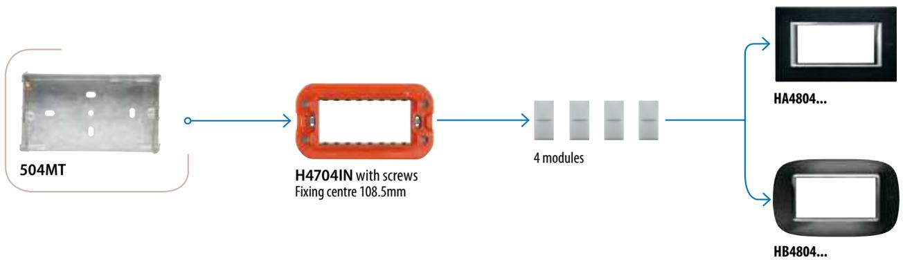
**NOTE:** the supporting frames are supplied with a pre-installed orange frame-cover and a transparent protection. It is recommended to remove the frame-covers before installing the plates. Devices available in white, tech and atrracite colour.
