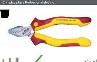
**Meets your requirements:** Safe pressing in marked trapezoidal/ semi-circular profiles. **Lowers your costs:** Durable thanks to highquality, chrome-plated plier surface to prevent corrosion. **Offers you full protection:** Each tool individually tested at 10,000 V AC and approved for 1,000 V AC. Crimping pliers Professional electric
